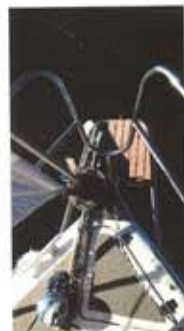
The upright on the port side of the bowsprit is for the bow light, which can be removed and stowed below
